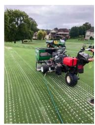
clean, precise channel of sand in the green to dilute our organic mat layer without having to pull a core of material out of the green which would take some time to heal. We can perform this less aggressive practice in the fall because we continue to receive the support to get very aggressive with organic matter removal in the spring. This process is
